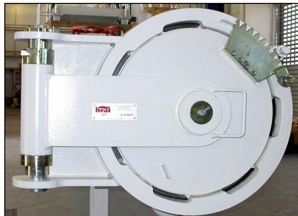
The second safety feature concerns the shape of the closing cap: the cap teeth are graded so that upon their engaging the cap is automatically placed at the correct distance to the flanged ring.
