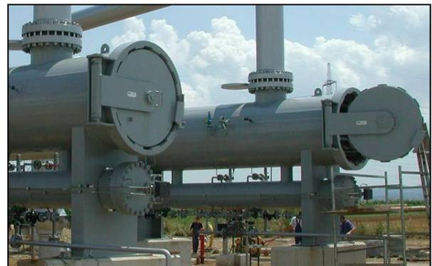
The flange ring is fitted with teeth (top left photo) designed to meet the requisite load-bearing capacity. A movable cap is opened and closed by a swivel arm attached to the flange ring. The cap is also fitted with teeth whose length, height and spacing match that of the outer teeth.
